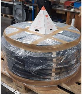
• The first layer must be between the first spool/coil and the pallet. If the weight is more than 40kg, the rings/coils must be further separated by appropriate intermediate layers.
